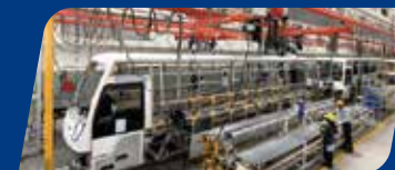
Structure Making Use of Jigs & Fixtures
