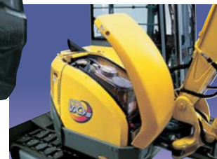
Battery, fuel and hydraulic oil can be checked more conveniently.
