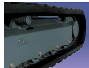
Angled crawler frame reduces unwanted build up of foreign matter.
