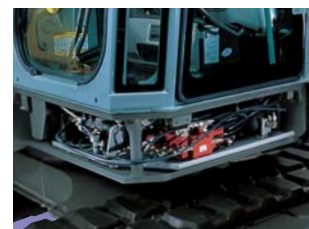
Removable side frame cover for easier service accessibility.
