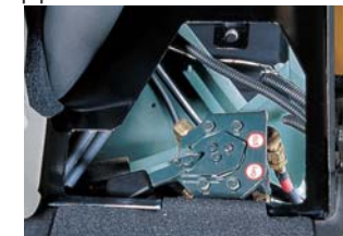
To enable the use of additional hydraulic attachments, PTO is piped to the end of the arm.
