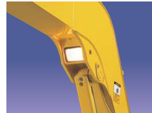
Integrated boom-light is protected from damage.
