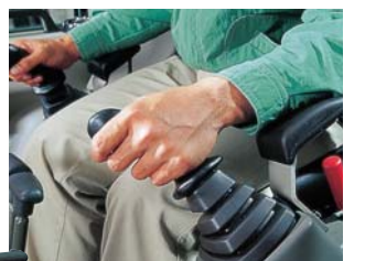
Joystick pilot controls and arm rests are convenient to use and reduce operator fatigue.
