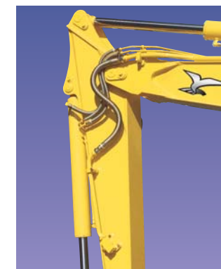
To enable the use of additional hydraulic attachments, PTO is piped to the end of the arm.
