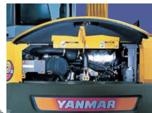
Large opening rear hood for easier maintenance.
