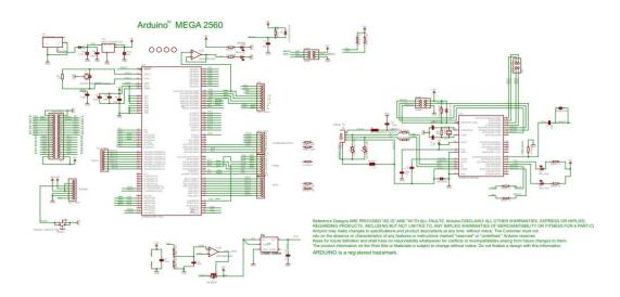
The schematic diagram of ATmel MCU ATMEGA16U2 MEGA 2560 R3 Improved Version CH340G Board is as shown in fig.
