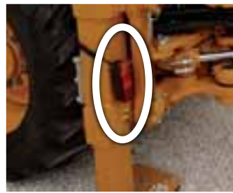
Rear road lights can be fitted on the stabilizer legs while traveling and on the cab when digging, providing maximum visibility and protection
